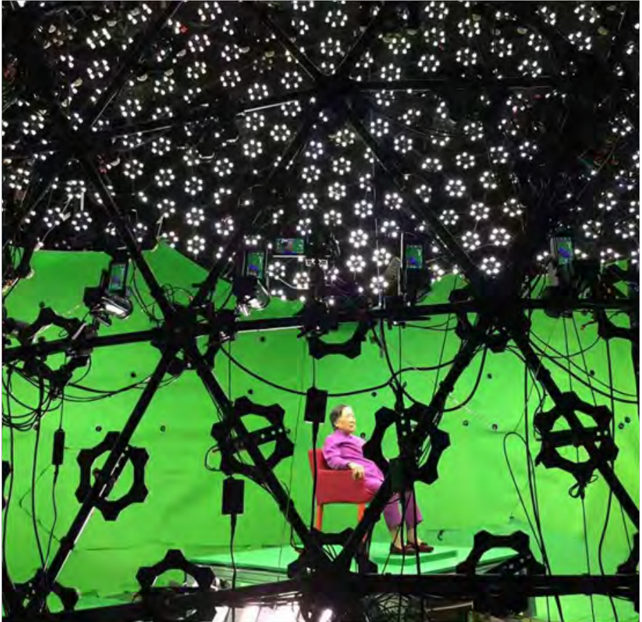
Figure 8. Xia Shuqin in Light Stage 6 Los Angeles October 2016. The interviewer sits outside of the stage with direct eye contact with the interviewee. The subject was illuminated by 3,000 individual LED lights. Credit: USC Shoah Foundation
